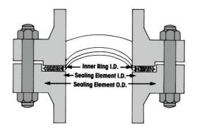
Standard 'RIR' gaskets are manufactured to 0.125" (3.2mm) thickness. The gasket features a solid metal inner ring nominally 0.090" (2.3mm) thick, as an integrated part of its design. The inner ring provides a positive stop preventing the gasket from over compression and possible damage.
