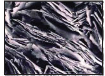
Vermiculite’s thin, flexible, soft plates can be exfoliated like graphite. They retain the sealability and low porosity of graphite, but Flexitallic’s new Thermiculite® sheet gaskets will not oxidize at high temperatures.
