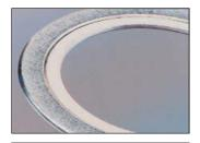
Style RIR - Solid inner metal ring acts as a compression stop and fills the annular space between flange bore and the inside diameter of the gasket. Designed to prevent accumulation of solids, reduce turbulent flow of process fluids and minimize erosion at flange faces. Suitable for male and female pipe flanges.
